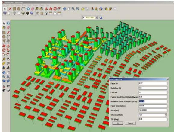
Figure 5 Solar radiation results displayed in SketchUp
