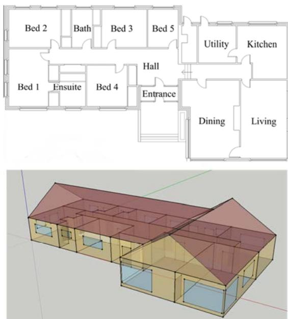
Figure 2: Single-storey detached house and thermal zones
