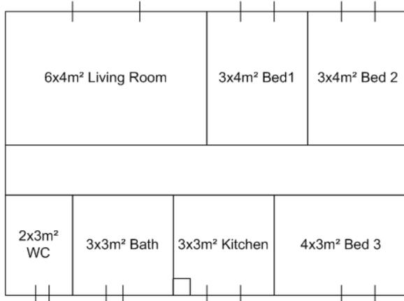
Figure 1: scheme of the internal architecture of the 84 m<sup>2</sup> dwellings
