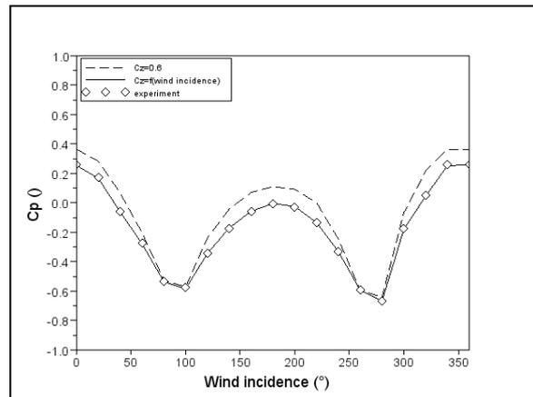
Figure 7 : evolution as function of wind incidence of the internal pressure coefficient  $C_p$  in the living room of floor 2 with and without optimisation of  $C_z$
