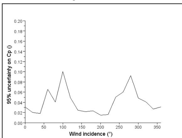
Figure 5: Pressure coefficient measurement uncertainty on a 95% interval confidence plotted as function of wind incidence
