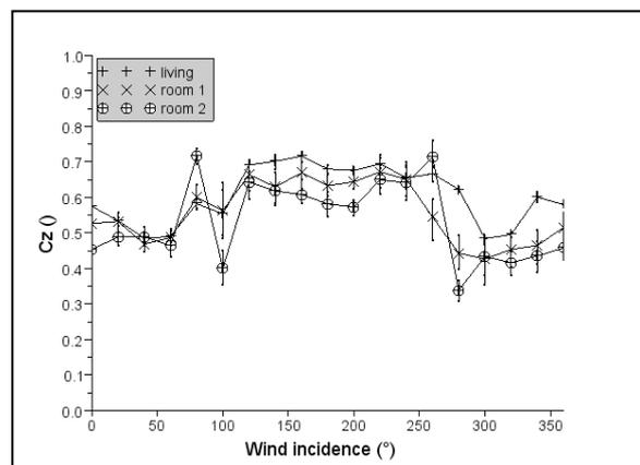
Figure 8:  $C_z$  coefficient as function of wind incidence for openings facing the direction  $0^\circ$  at floor 2
