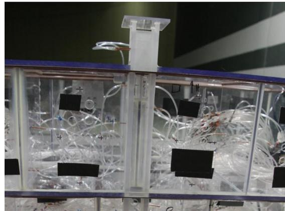
Figure 4: detailed view of the collective duct and static extractor
