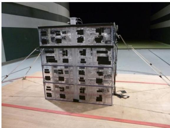
Figure 3: view of the building inside the wind tunnel
