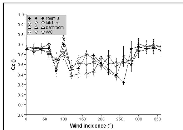
Figure 9:  $C_z$  coefficient as function of wind incidence for openings facing the direction  $180^\circ$  at floor 2
