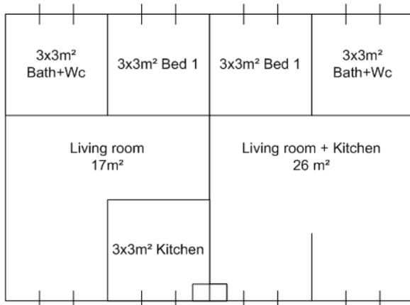
Figure 2: scheme of the internal architecture of the two 42 m<sup>2</sup> dwellings
