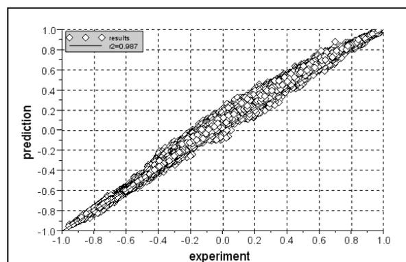
Figure 6: correlation between predicted and measured internal pressure coefficient  $C_p$  for all the rooms and configurations with a constant value of  $C_z=0.6$
