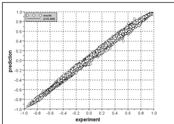
Figure 10: correlation between predicted and measured internal pressure coefficient  $C_p$  for all the rooms and configurations with optimized  $C_z$  variation laws
