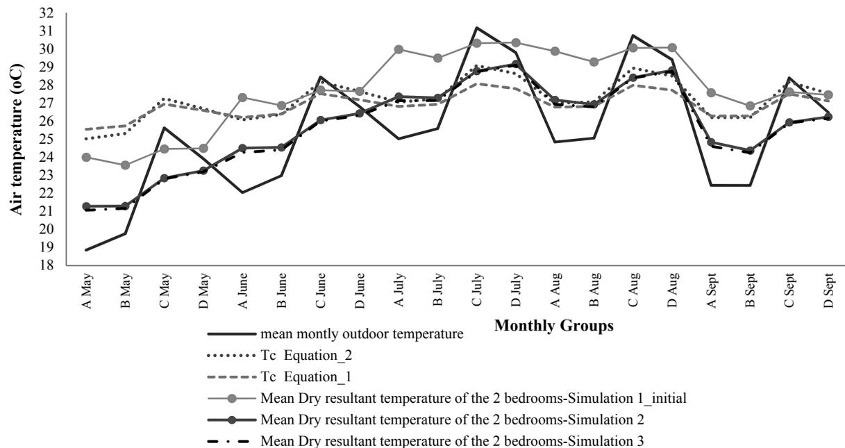
Figure 5 External air temperature, comfort temperatures and internal dry resultant temperatures before and after the changes in the cooling strategy.
