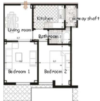
Figure 3 Floor Plan of case study apartment
