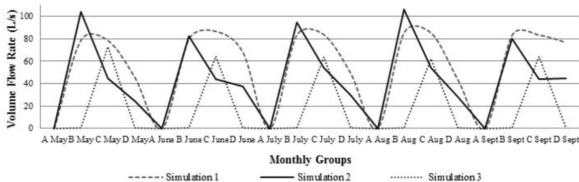
Figure 6 Mean volume flow rate through the openings on the external wall subdivided by group of time for the different simulations results
