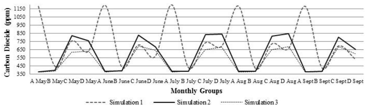
Figure 7 Mean value of the carbon dioxide concentration in ppm of the 2 bedrooms for the examined period, subdivided by group of time for the different simulations results
