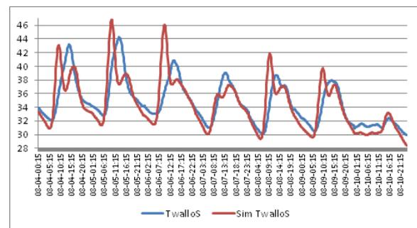
Figure 3: Comparison of outside wall temperature between simulated and sensor data
