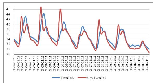
Figure 5: Comparison of zone temperature between simulated and sensor data during calibration procedure
