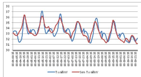
Figure 4: Comparison of inside wall temperature between simulated and sensor data
