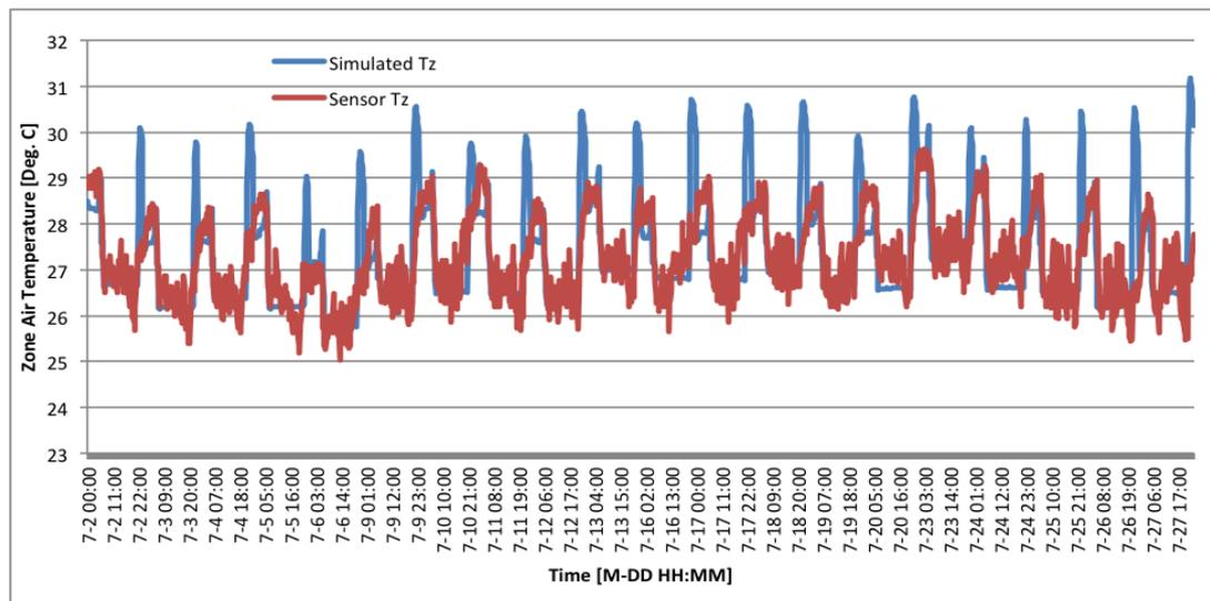
Figure 6: Comparison between computed and actual zone air temperature (July 02-July27, weekdays)
