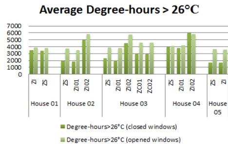
Figure 1 - Average Degree-hours >26°C per zone for both closed and opened windows conditions.
