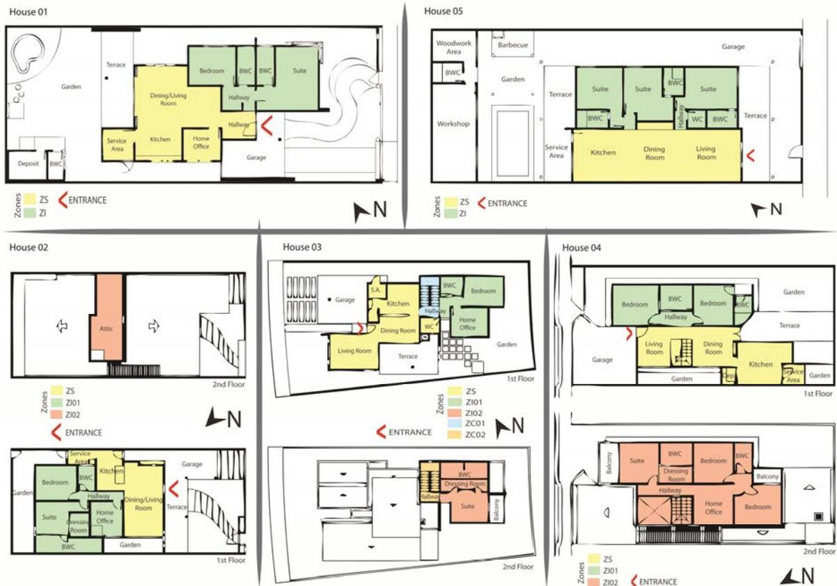
Figure 12 – All houses' floor plans with its respective orientations and zones.
