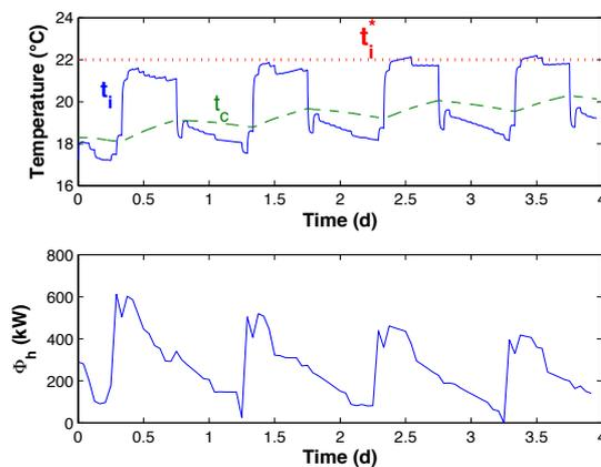
Figure 6: MPC control: evolution of the state variables and of the setpoint (upper) and of the control variable  $\Phi_h$  (lower)
