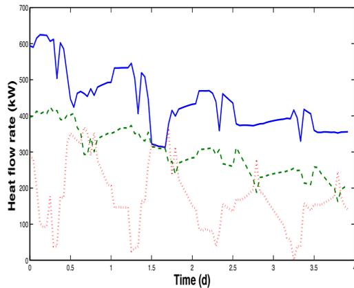
Figure 5: MPC strategy: predicted profile of the control variable (solid: morning, dashed: afternoon, dotted: night)
