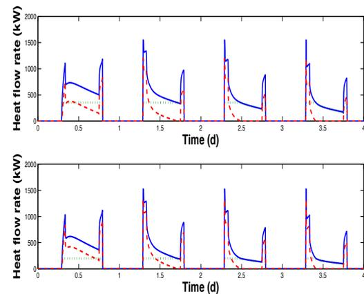
Figure 4: PI-control: total and per source heat flow rates (upper: net heat flow rates, lower: primary heat flow rates; solid: total, dashed: boiler, dotted: heat pump)
