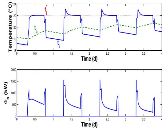
Figure 3: PI-control: evolution of the state variables and of the setpoint (upper) and of the control variable  $\Phi_h$  (lower)
