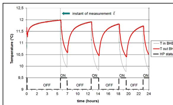
Figure 5 Case study: evaluation of the average ground temperature after an operation of one year
