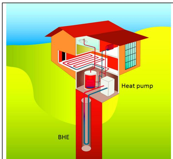
Figure 1 Scheme of a GSHP with vertical BHE
