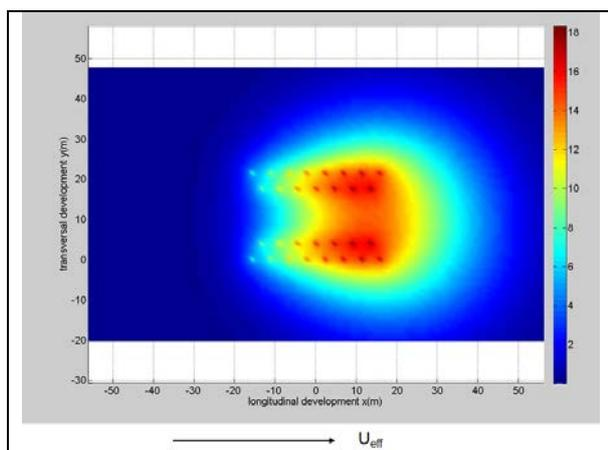
Figure 7 Simultaneous operation of the twin blocks - Ground temperature decrease after 10 years
