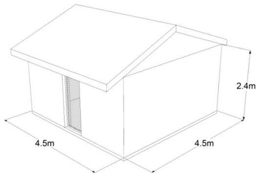
Figure 1 Diagram of the test cell configuration
