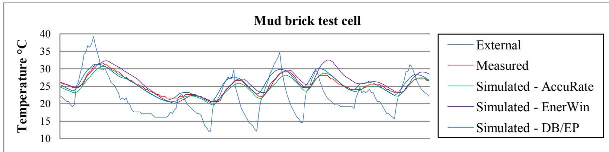
Figure 5 Mud brick test cell measured and predicted indoor temperatures from 14<sup>th</sup> – 21<sup>st</sup> December 2006
