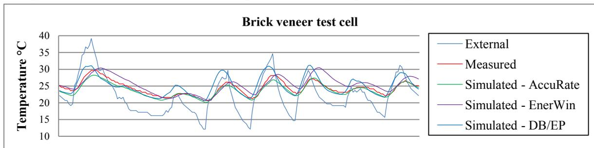
Figure 6 Brick veneer test cell measured and predicted indoor temperatures from 14<sup>th</sup> – 21<sup>st</sup> December 2006
