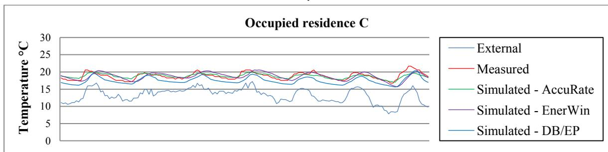
Figure 9 Occupied residence C Living/kitchen area measured and predicted indoor temperatures from 10<sup>th</sup> – 16<sup>th</sup> May 2011
