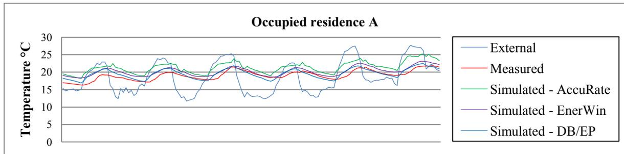
Figure 7 Occupied residence A Living/kitchen area measured and predicted indoor temperatures from 12<sup>th</sup> – 18<sup>th</sup> April 2012
