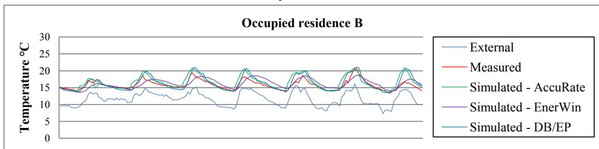
Figure 8 Occupied residence B Living/kitchen area measured and predicted indoor temperatures from 25<sup>th</sup> – 31<sup>st</sup> May 2011
