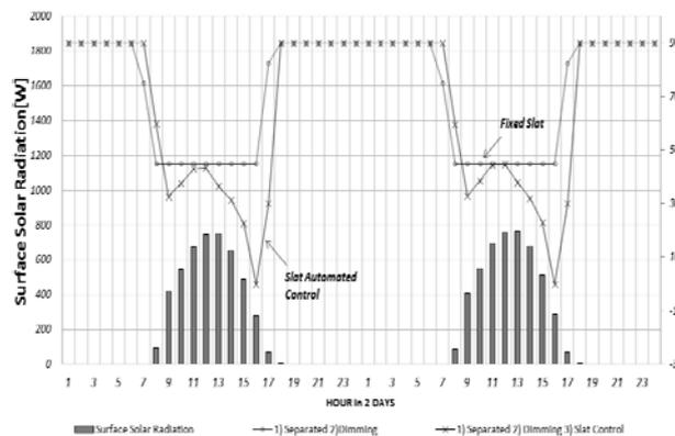
Figure 6. Slat angle variation in the typical winter days (Jan. 30<sup>th</sup> ~ 31<sup>st</sup>) (Oh 2011, 2012)
