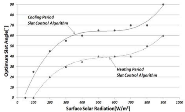
Figure 3. Slat angle control algorithm in heating and cooling modes (Oh 2011, 2012)
