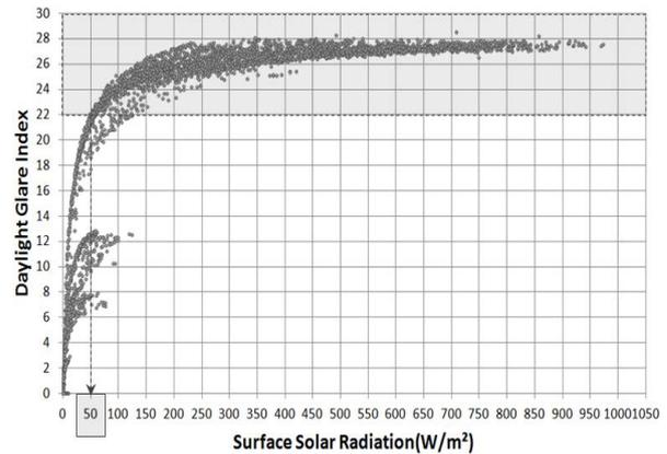
Figure 4. DGI analysis in each vertical solar radiation without blind operation (Oh 2011, 2012)
