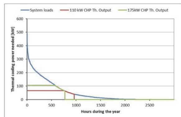
Figure 6 – Cooling thermal production of the two different CCHP units considered
