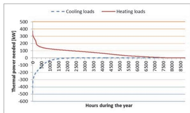
Figure 4 – Total base case heating and cooling loads.
