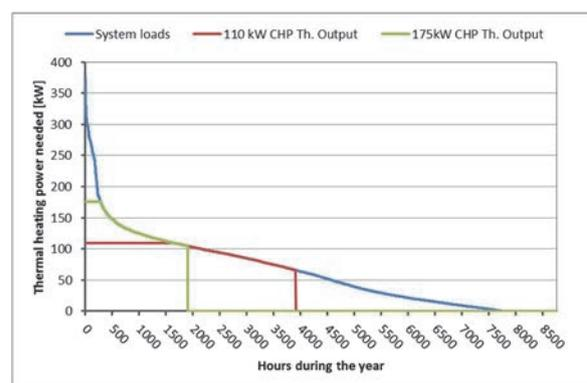
Figure 5 – Thermal power curve and area of operation of the CHP systems
