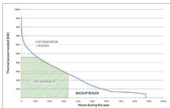
Figure 3 – Example of a thermal power curve and area of operation of the cogeneration system
