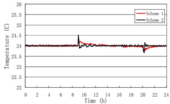
Fig.4 Temperature in exhibition room of two schemes on the test day
