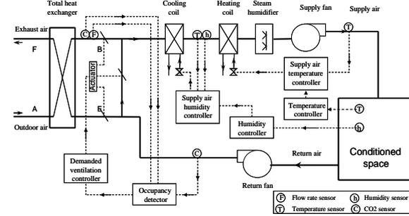
Fig.1 The CAV system with separate temperature and humidity controls by cooling-reheating
