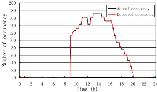
Fig.6 Comparison between actual occupancy and detected occupancy
