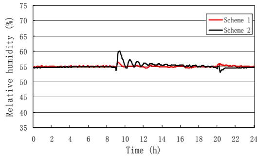
Fig.5 Relative humidity of exhibition for two schemes on the test day
