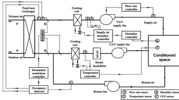
Fig.2 The DOAS-integrated system with decoupling control strategies for museums
