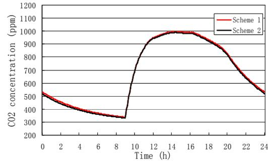
Fig.7 CO<sub>2</sub> concentrations of exhibition for two schemes on the test day
