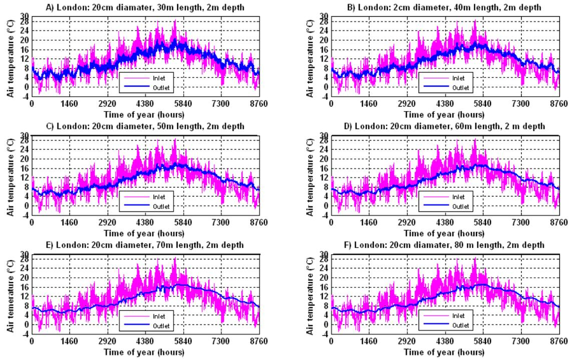
Figure 2 Inlet and Outlet air temperature profile for 20 cm diameter EAHX, London
