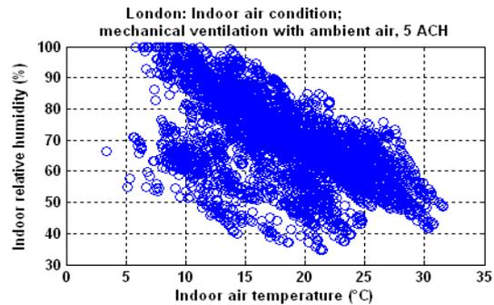
Figure 8 London: Indoor condition for ventilation with ambient air, 4 & 5 room air changes per hour (ACH)
