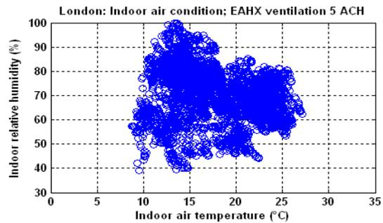
Figure 9 London: Indoor condition; EAHX ventilation 0.3m diameter, 60m length and 4 & 5 room air changes
