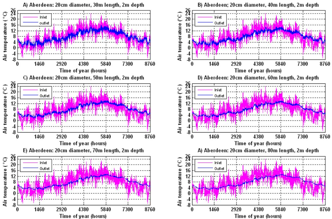
Figure 3 Inlet and outlet air temperature for 20cm diameter EAHX in Aberdeen
