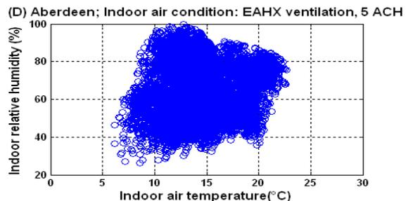
Figure 11 Aberdeen; Indoor condition, EAHX ventilation 30cm diameter, 60m length and 4-5 air changes (ACH)
