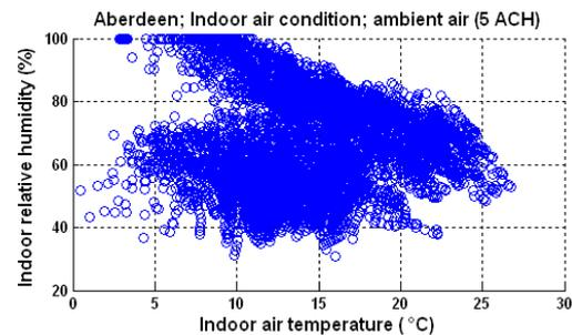
Figure 10 Aberdeen: Indoor air condition for ventilation with ambient air, 4-5 Air changes (ACH)
