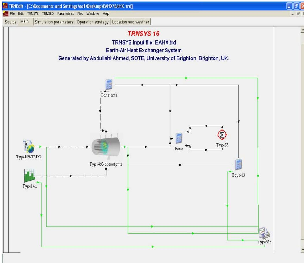
Figure 1 TRNSYS earth-air heat exchanger simulation tool
