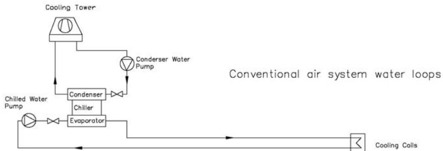
Figure 4 Radiant cooling with DOAS system and VAV system configurations (water side)
