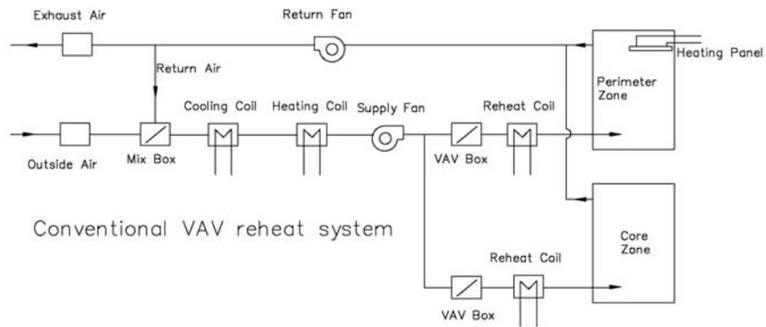
Figure 3 Radiant cooling with DOAS system and VAV system configurations (air side)
