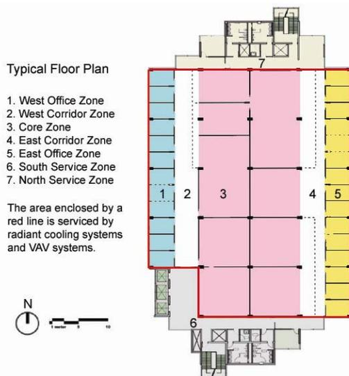
Figure 1 Typical floor plan, levels 3 to 7
