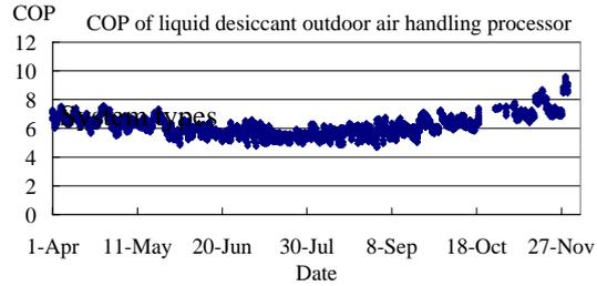
Figure 9.4 Hourly COP of THICS liquid desiccant outdoor air handling processor-GZ
