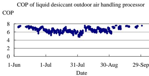
Figure 9.1 Hourly COP of THICS liquid desiccant outdoor air handling processor-BJ
