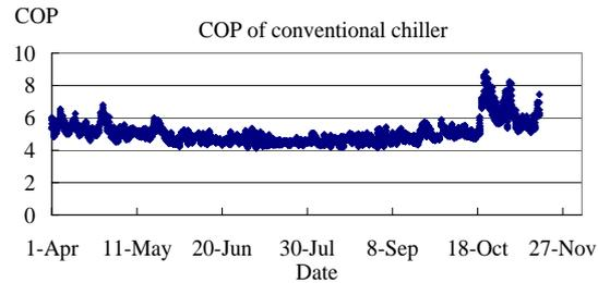
Figure 9.5 Hourly COP of THICS high temperature water chiller-GZ
