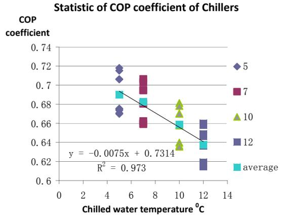
Figure 4 Statistic of COP coefficient  $\eta$  of chillers
