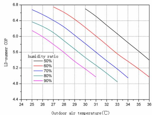
Figure 5 Summer COP of liquid desiccant outdoor air handling processor
