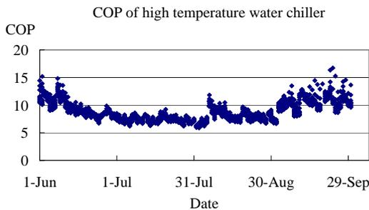
Figure 9.2 Hourly COP of THICS high temperature water chiller-BJ
