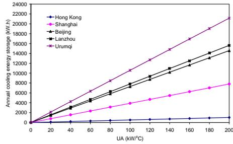
Fig.3. Annual cooling energy storage by the evaporative cooling at different UAs
