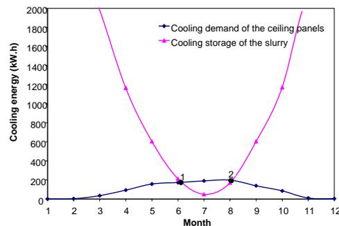
Fig. 7. Comparison of the cooling energy storage and cooling demand of the ceiling panels in Urumqi
