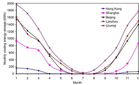
Fig.4. Monthly cooling energy storage by the evaporative cooling at UA=100 kW/°C
