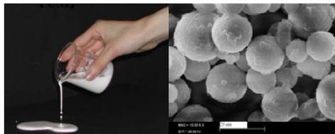
Fig.1. Appearance of the MPCM slurry and SEM microscopic image of the MPCM particles
