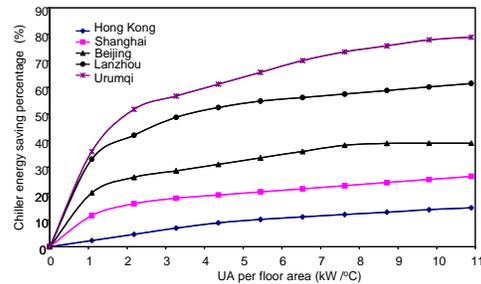
Fig. 6. Chiller energy saving percentage with different heat exchanger sizes
