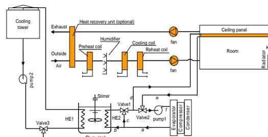
Fig.2. Schematic diagram of the hybrid system
