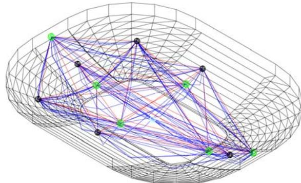
**Figure 10** Image of the direct (**Red**) and 1st reflected (**Blue**) sound rays showing the simulated crowd noise for various locations.
