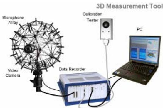
**Figure 1.** Acoustic Camera recording system
