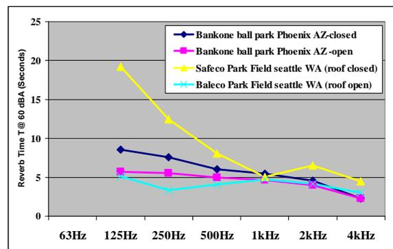
**Figure 7** RTs 60 dBA based on measured data for existing stadiums with their roof top open and closed.
