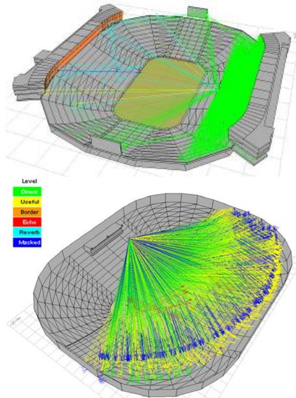
**Figure 9** Simulation of the open top stadium with and without the new sky boxes
