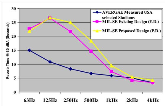
**Figure 8** RTs 60 dBA based simulation data for existing stadiums and the proposed new skyboxes
