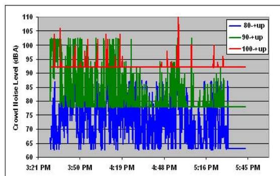
**Figure 5** A time series measured data in the stadium for crowd noise at 80 dBA, 90 dBA, and 100 dBA and up
