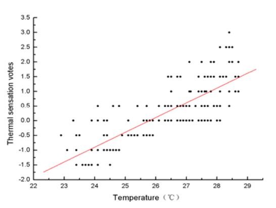
Figure 11 Calculation of thermal neutral temperatures in summer conditions
