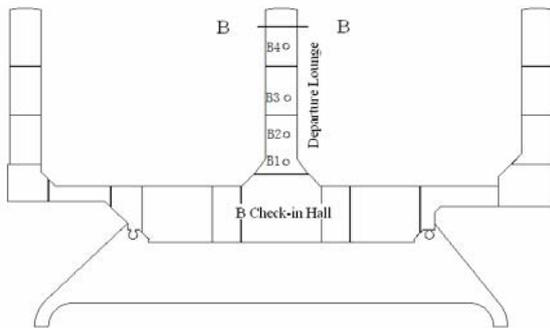
Figure 3 Indoor Measurement Points of Terminal Building
