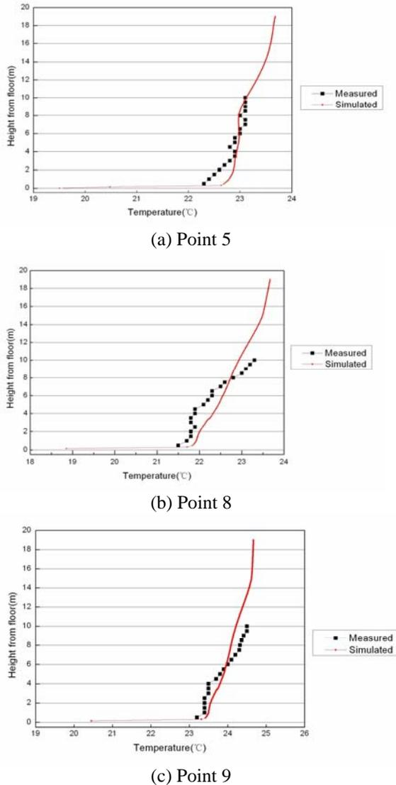
Figure 12 Compared CFD results with measurement results of vertical air temperature profiles
