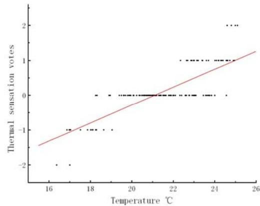
Figure 10 Calculation of thermal neutral temperatures in winter conditions
