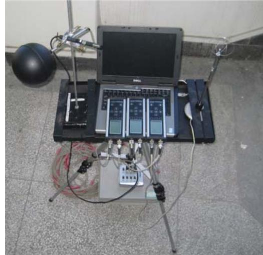
Figure 5 Thermal comfort meter
