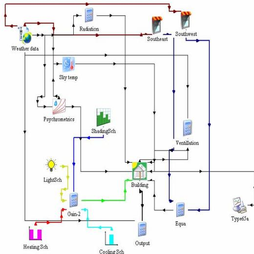
Figure 2: TRNSYS Model of the Net Zero Energy House.
