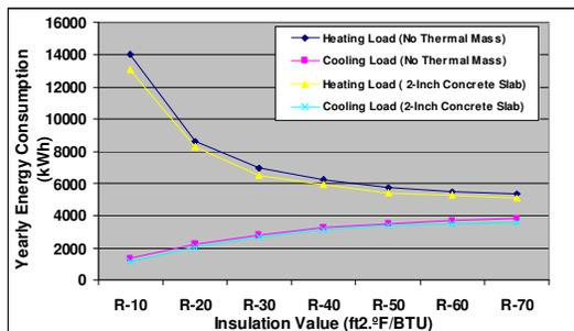
*Figure 8: Comparison of the impact on the heating and cooling loads as insulation levels are varied when thermal mass is used versus no thermal mass*
