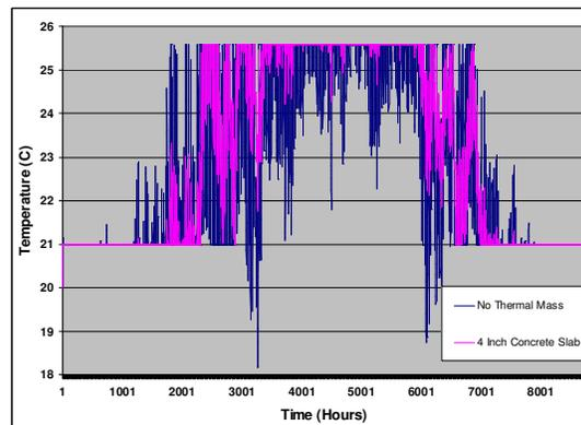
*Figure 9: Yearly temperature profile of the Mezzanine Floor of the house comparing the impact of using a 4-inch thick concrete slab.*
