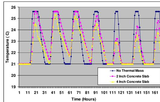
Figure 4: Temperature profile of the 3<sup>rd</sup> floor of the Net Zero Energy house during a typical winter week with varying thermal mass
