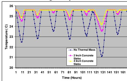
Figure 6: Temperature profile of the 3<sup>rd</sup> floor of the Net Zero Energy house during a typical summer week with varying thermal mass
