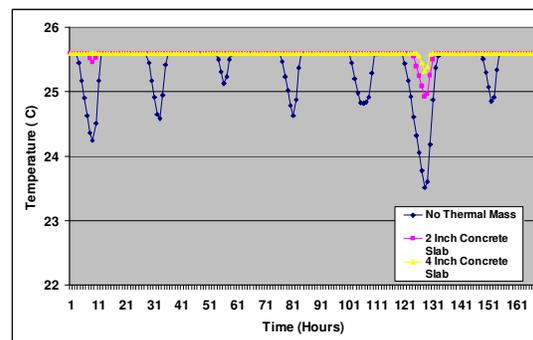
Figure 5: Temperature profile of the Mezzanine floor of the Net Zero Energy house during a typical summer week with varying thermal mass
