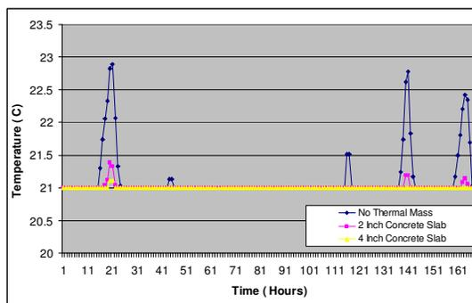
Figure 3: Temperature profile of the Mezzanine floor of the Net Zero Energy house during a typical winter week with varying thermal mass
