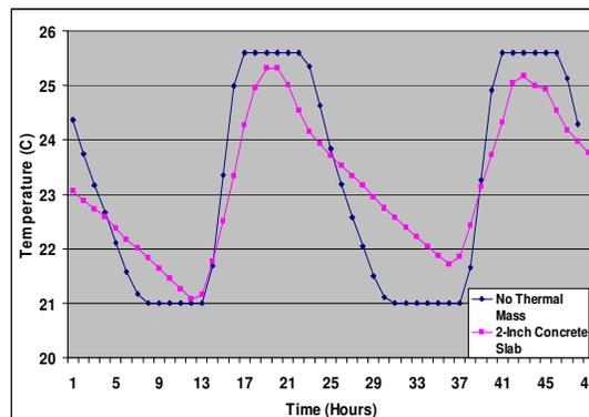
*Figure 10: Temperature profile of the 3rd Floor of the house for a 48-hour duration for the winter season,, comparing the impact of using a 4-inch thick concrete slab*
