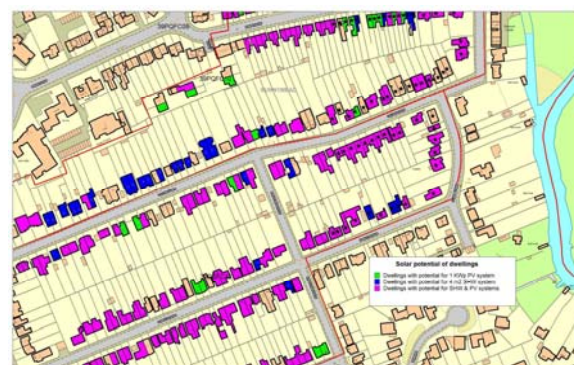
Figure 4 Estimating the solar potential of dwellings in North Oxford using DECoRuM
