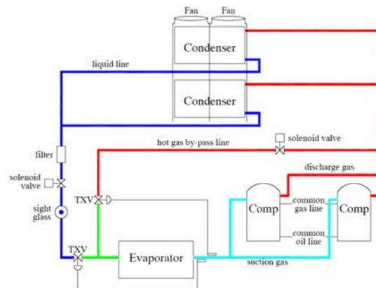
Figure 3: Air-cooled chiller refrigeration circuit
