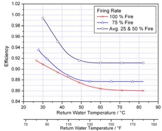
Figure 6: Efficiency curves of the boiler
