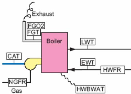
Figure 5: Scheme of the condensing boiler with measuring points
