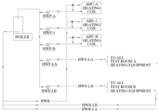
Figure 4: Simplified heating water piping schematic
