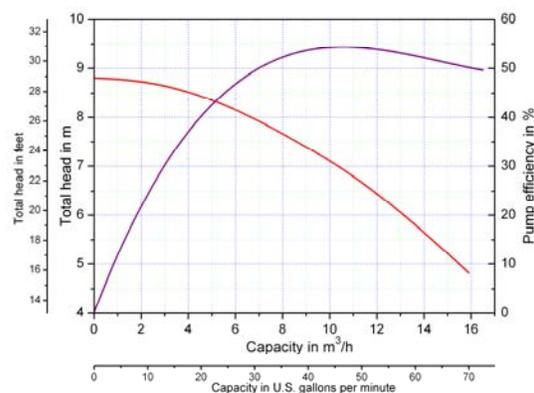
Figure 8: Heating water pump performance curve extract
