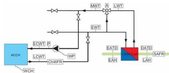
*Figure 1: Scheme of the chilled water system with measuring points*
