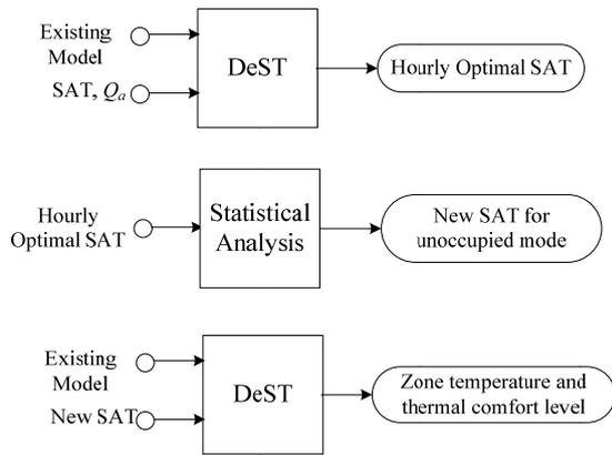
Figure 6 Inputs and outputs in SAT optimization
