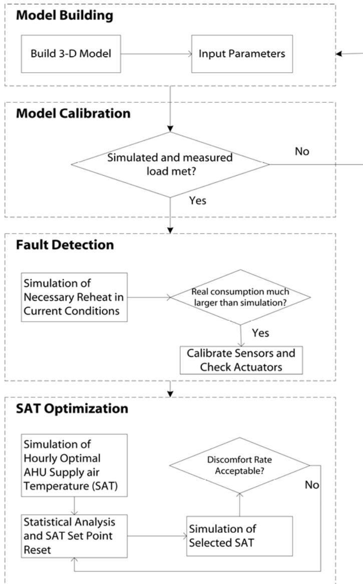
Figure 1 Process of using simulation in diagnosis of AHU VAV system
