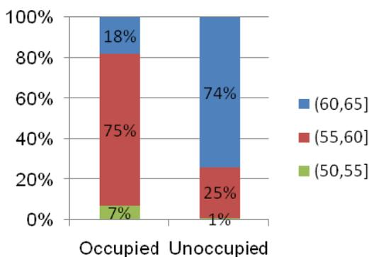
Figure 8 Analysis of AHU supply-air temperature in summer conditions
