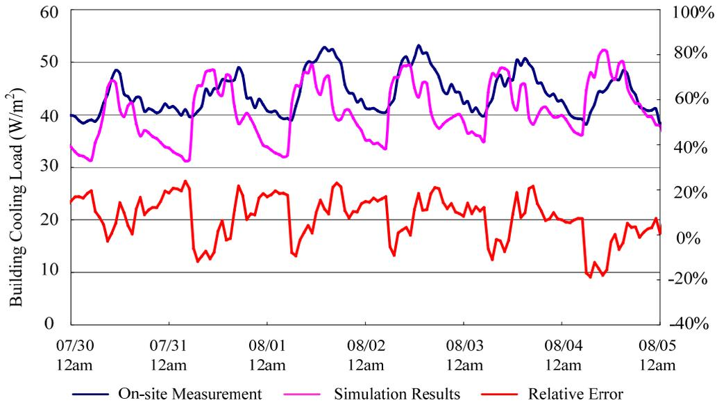
Figure 3 Comparison of building cooling load of on-site measurements and simulation results
