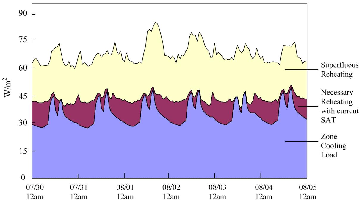
Figure 5 Simulation results of zone cooling load, necessary reheating with current SAT and superfluous reheating of one AHU
