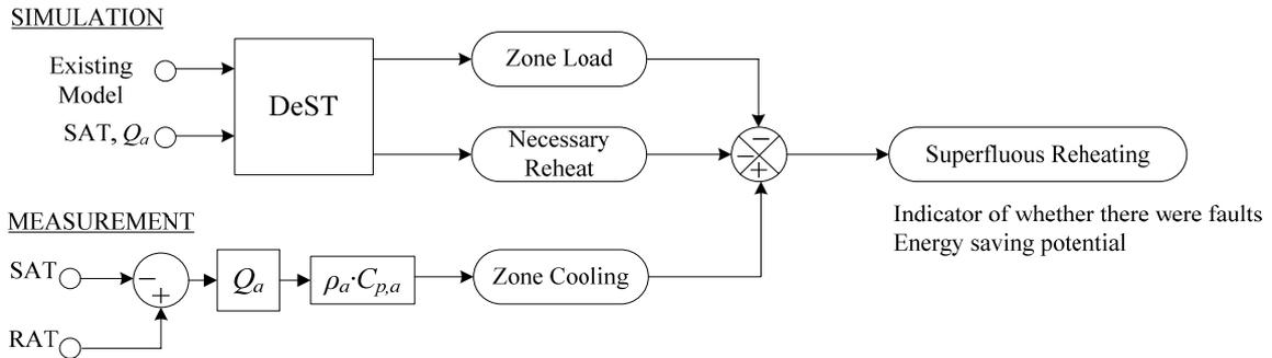
Figure 4 Block diagram of fault detection
