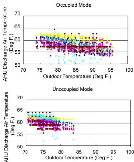
Figure 7 Optimal AHU supply-air temperature by simulating
