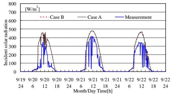
Figure 12 Incident total solar radiation on south window of the living room, Sep.20-Sep.22
