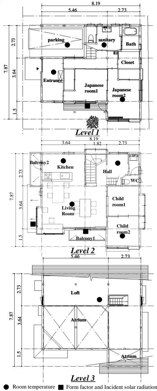
Figure 3 Plan and Measuring point
