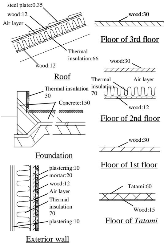
Figure 4 Composition of walls (Unit: mm)
