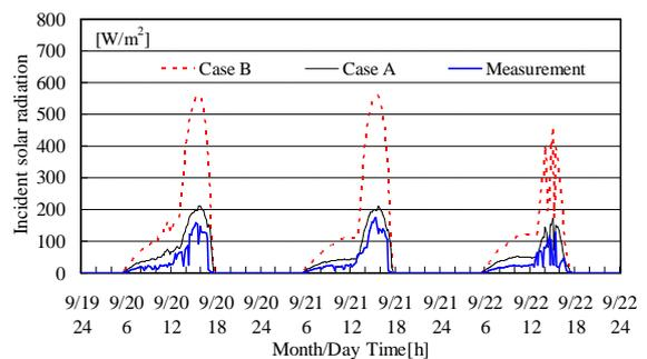
Figure 13 Incident total solar radiation on west window of the living room, Sep.20-Sep.22
