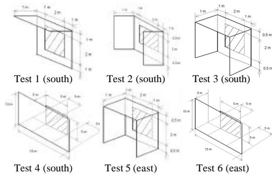
Figure 5 Test cases acc. to DIN EN ISO 13791- 7.2.4
