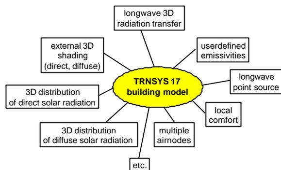
*Figure 1 New features of the multizone building model*
