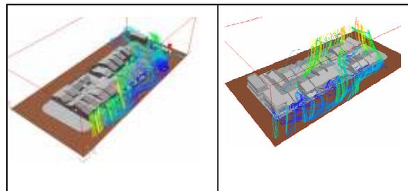
Figure 7 Streamlines for houses facing prevailing SE winds.
