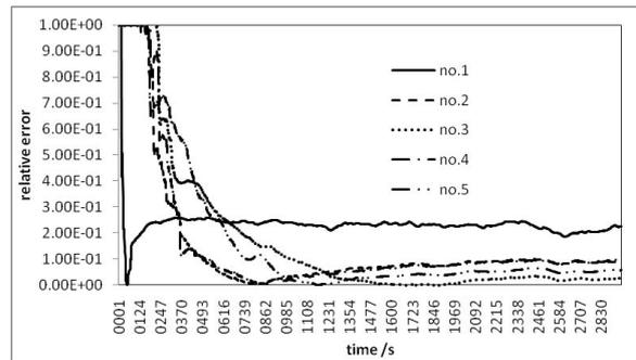
Fig.7 Relative error of CO<sub>2</sub> concentrations between test and calculation
