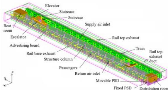
Figure 2 Three-dimensional model of subway island platform
