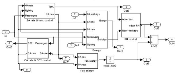
Figure 6 The DCV system control model
