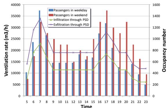
Figure 8 Variation of passengers, infiltration and exfiltration rate through PSDs
