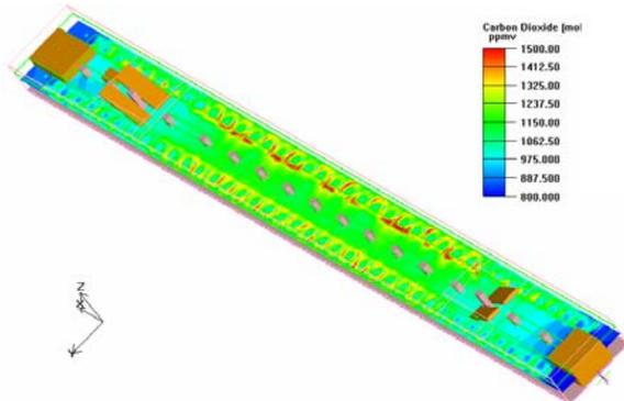
Figure 3 CO<sub>2</sub> concentration distribution at the height of 1.65m above the platform
