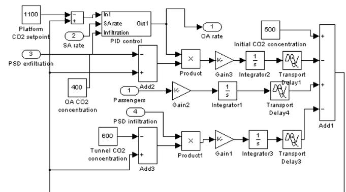
Figure 4 CO<sub>2</sub> control sub-model
