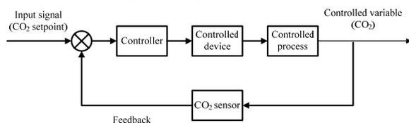
Figure 1 Control diagram for DCV system
