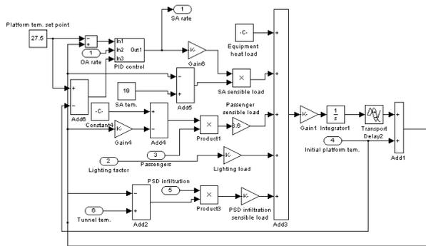
Figure 5 Temperature control sub-model
