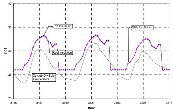
Figure 7 Temperature profile of upper floor
