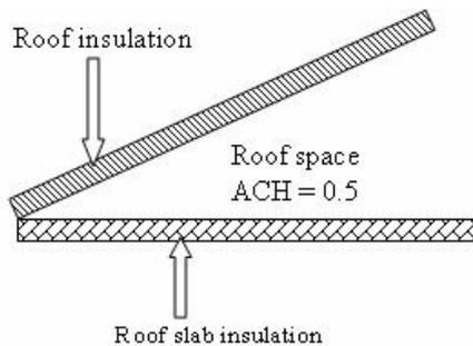
Figure 5 Roof insulation installation.
