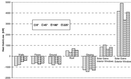
Figure 11 Comparison of heat transfer through building envelopes for different building orientation
