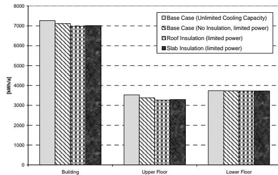
Figure 13 Comparison of annual cooling energy as the effect of limited power of the cooling device.
