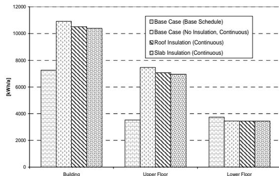
Figure 14 Comparison of annual cooling energy as the effect of operational time of the cooling device
