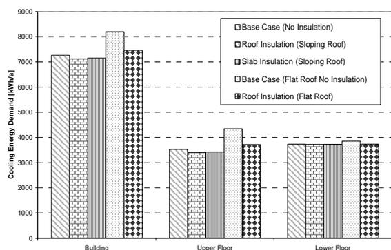
Figure 15 Comparison of annual cooling energy between sloping roof and flat roof
