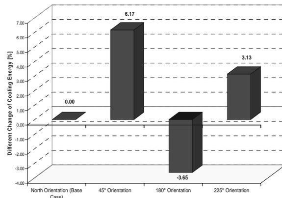
Figure 10 Effect of building's orientation to the cooling energy demand.
