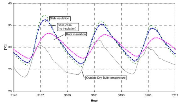
Figure 6 Temperature profile inside roof space
