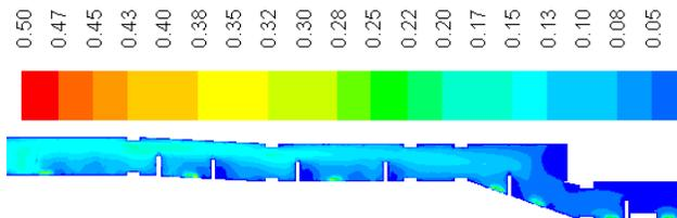
Figure 15 Predicted velocity Contours, m/s KV15
