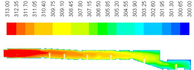
Figure 16 Predicted temperature Contours, K, KV15
