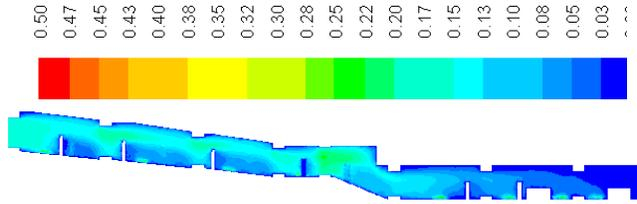
Figure 12 Predicted velocity Contours, m/s KV13
