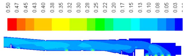
Figure 9 Predicted velocity Contours m/s, KV2
