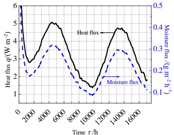
Figure 8 Variation of the heat and moisture flux on the wall of the earth-sheltered building
