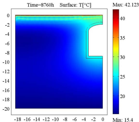
Figure 6 Temperature profile of the earth-sheltered building envelope and the surrounding soils at the time of 2 years
