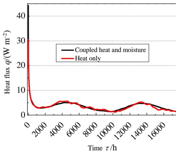
Figure 10 Comparison of the heat flux by the model in this paper and the heat transfer only model
