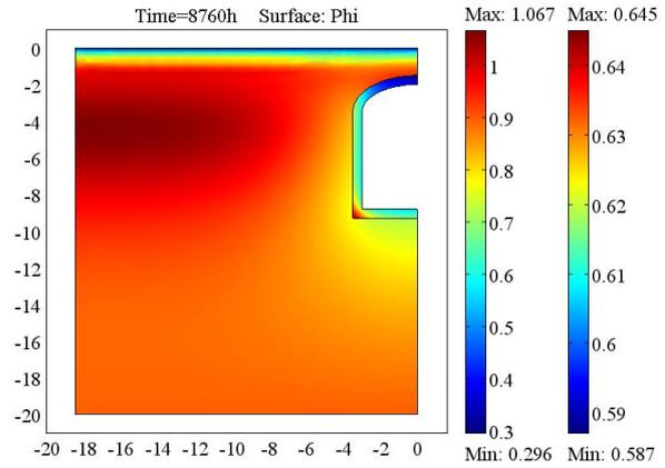
Figure 7 Relative humidity profile of the earth-sheltered building envelope and the surrounding soils at the time of 2 years
