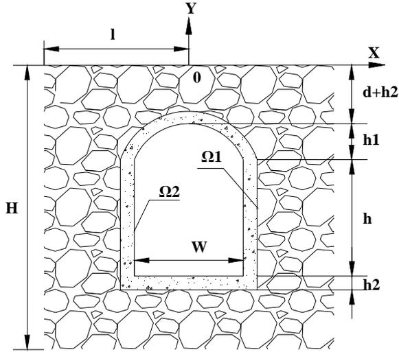
Figure 1 Cross-section of typical shallow buried underground engineering
