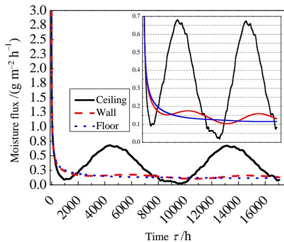
Figure 9 Variation of the moisture flux in the ceiling, floor and wall of the earth-sheltered building
