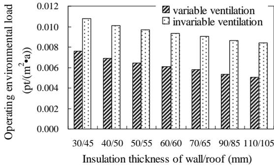
Figure 6-b operating environmental load
