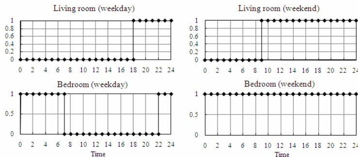
Figure 3 Operation schedules of air conditioners for intermittent heating and cooling
