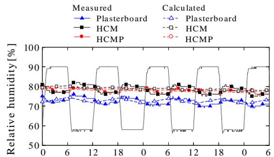
Figure 7 Measured and calculated relative humidity (54 hours after 3 days)
