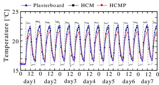
Figure 4 Air temperature in the model room
