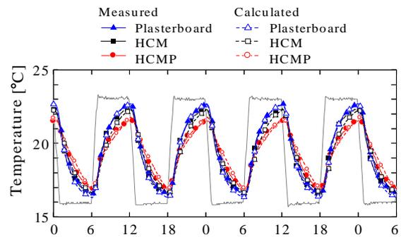
Figure 6 Measured and calculated air temperature (54 hours after 3 days)
