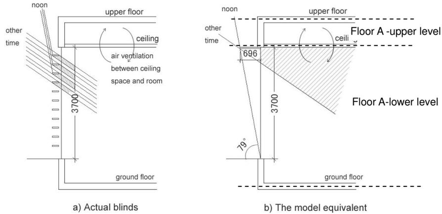
Fig 2. The blinds with horizontal slates and the overhang with equivalent shading effect.
