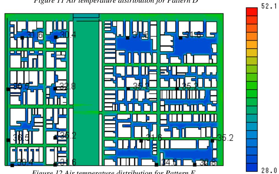
Figure 12 Air temperature distribution for Pattern E
