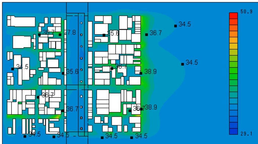
Figure 8 Air temperature distribution for Pattern A
