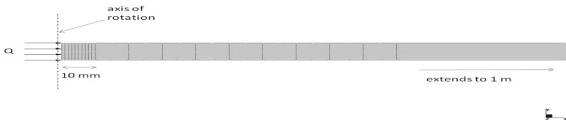
Fig. 3: Axisymmetric representation of material surrounding thermal probe. The model comprises 24 quadrilateral elements and 123 nodes.
