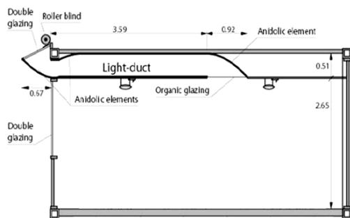
c). Cross-section of Anidolic duct in a room
