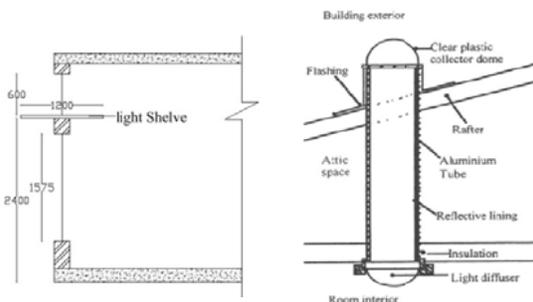
a). Cross-section of Light shelf      b). Cross-section of Light tubes
