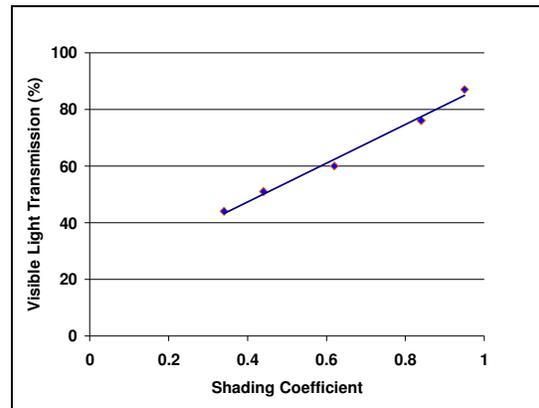
**Figure 6: Relationship between shading coefficient and visible light transmittance for the glazing selected.**
