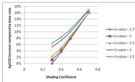
**Figure 8: Comparison of emissions with base case depending on variations of shading coefficient and U-Value of the glazing with vertical fins.**
