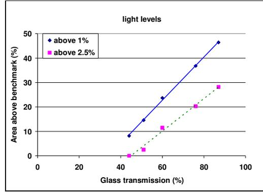
**Figure 10: Comparison of area above the 1% and 2.5% daylight factor threshold and the glazing transmission.**
