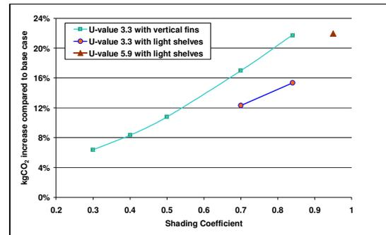
**Figure 14: Comparison of emissions with base case depending on variations of shading coefficient and U-Value of the glazing and addition of light shelves**
