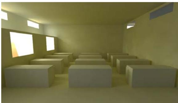
Figure 6 Three dimensional picture of a classroom for 25 students with projected clerestory is resulted by Radiance (link to Ecotect) simulation.
