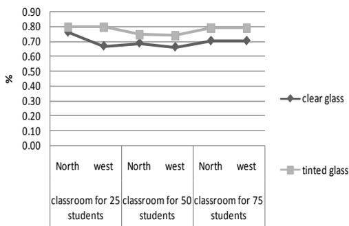
Figure 13 Comparison of daylight distribution between projected clerestory window with clear glass and with tinted glass
