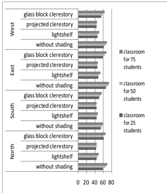
Figure 2 Hourly Thermal Transfer Value ( $W/m^2$ ) of Window with 34-39% WWR
