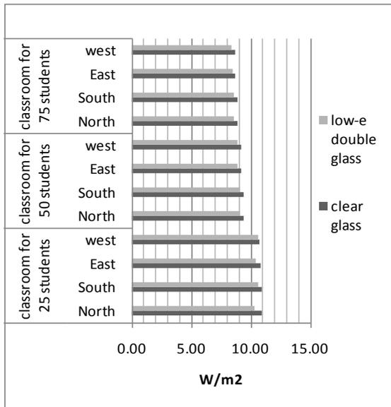
Figure 11 Comparison of Hourly heat gains through the building fabrics between projected clerestory with single glazing and with low-e double glazing
