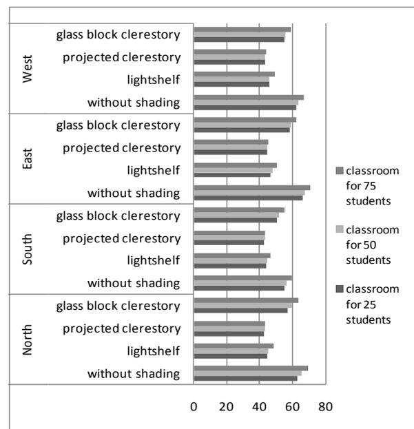
Figure 3 Hourly Thermal Transfer Value ( $W/m^2$ ) of Window with 20% WWR
