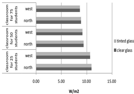
Figure 12 Comparison of hourly heat gains through the building fabrics between projected clerestory window with clear glass and with tinted glass
