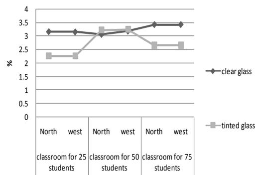
Figure 10 Comparison of average daylight factor between projected clerestory window with clear glass and with tinted glass
