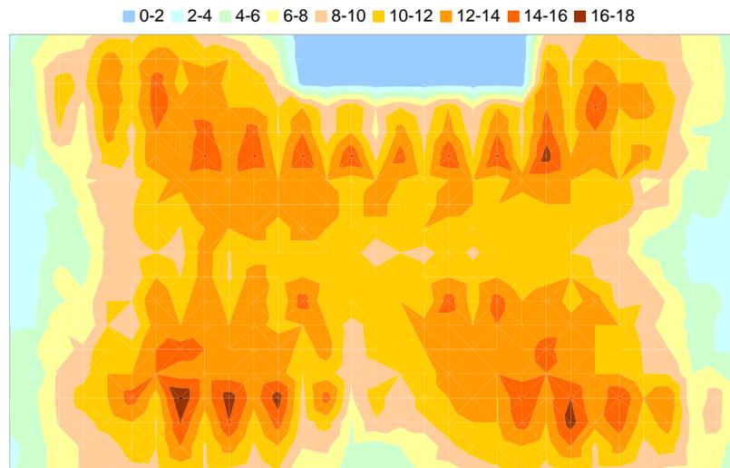
Figure 3 Daylight factor distributions on the floor of the building
