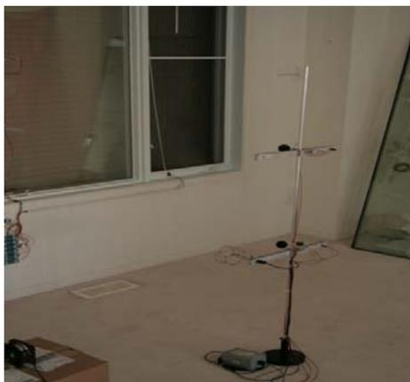
Figure 3 Probes for thermal and air measurements (air temperature and velocity, globe temperature and illuminance) near the south-facing window
