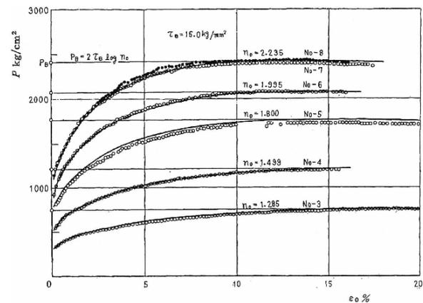
Figure 4 The relation between the distortion on outside radius of brass tube and limit pressure inside brass tube
