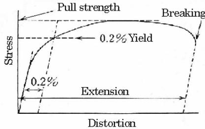
Figure 2 Stress-strain diagram of nonferrous metals material
