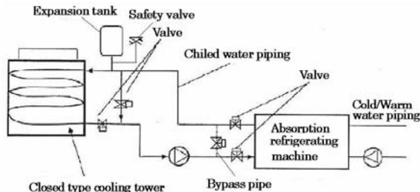
Figure 5 The heat source system which possesses object closed type cooling tower
