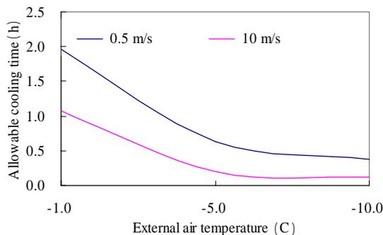
Figure 6 Relation between external air temperature/wind velocity and allowable cooling time
