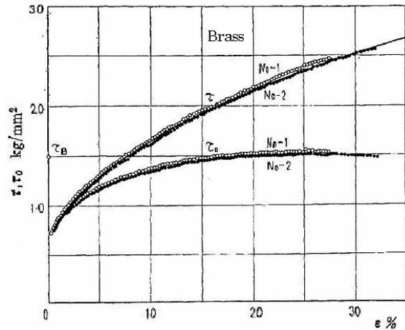
Figure 3 The relation between the distortion and the straightening shearing stress on inside radius of the brass tube
