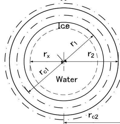
Figure 1 Computation model allowable freezing quantity in tube
