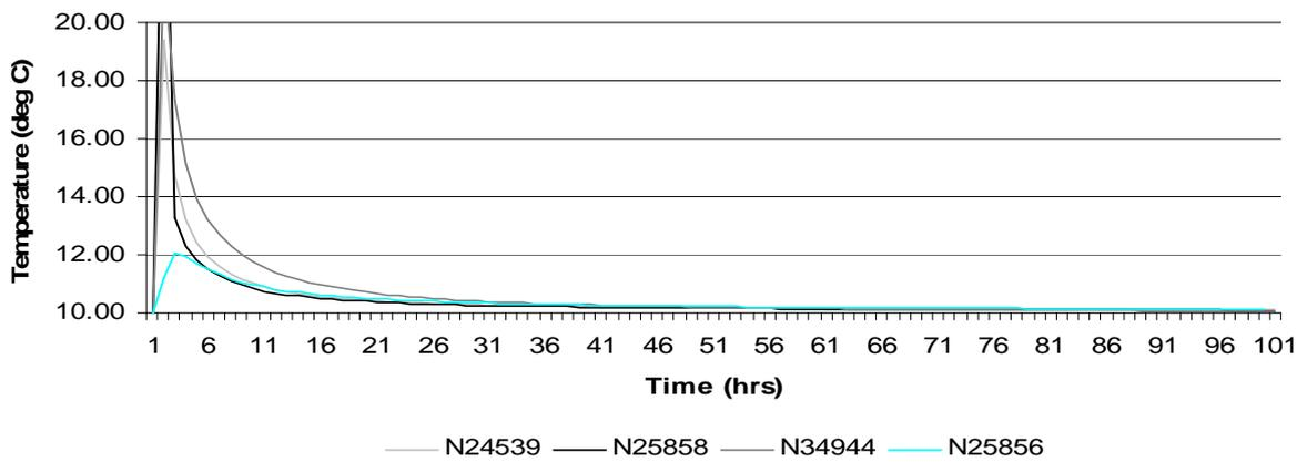
Figure 4 Temperature response factors at the three grid nodes due to an internal radiant or air point temperature excitation
