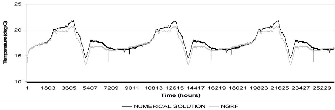
Figure 6 Temperature prediction at grid node 24539 with the use of 1000 hours of the time series responses
