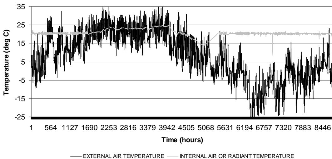
Figure 2 Boundary temperature conditions
