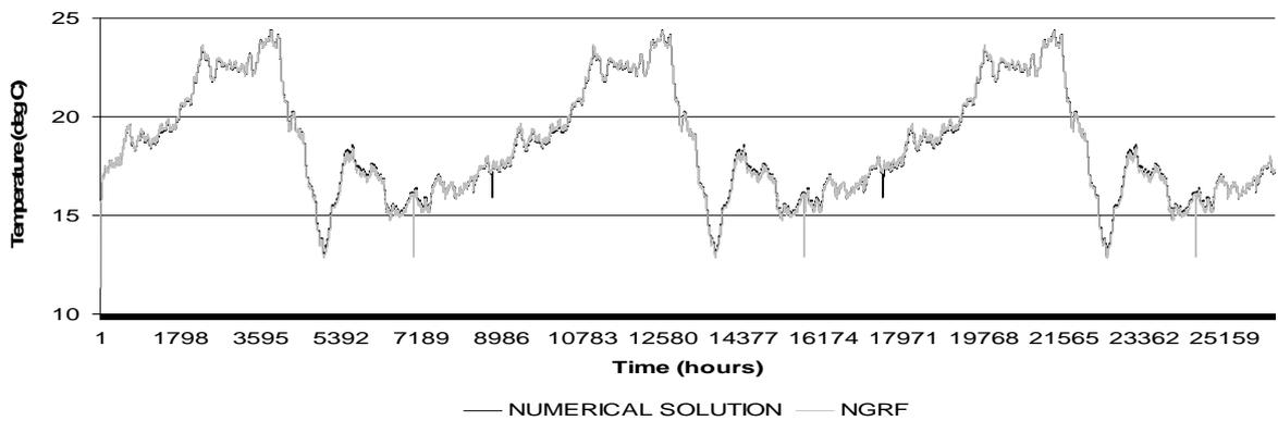
Figure 5 Temperature prediction at grid node 34944 with the use of 1000 hours of the time series responses
