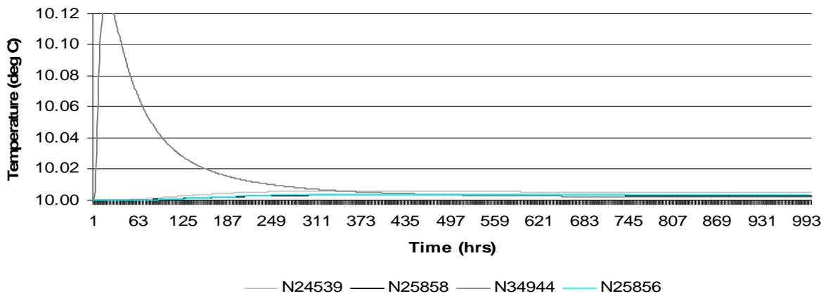
Figure 3 Temperature response factors at the four grid nodes due to an external temperature excitation
