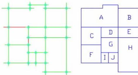
Figure 13 Arrangement of segment lines formed from two sets of contour lines used for recognition of elementary fragments of floor separating adjacent spaces.
