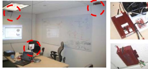
Figure 4 Test-bed in a conference room, wireless mote and occupancy counting input device
