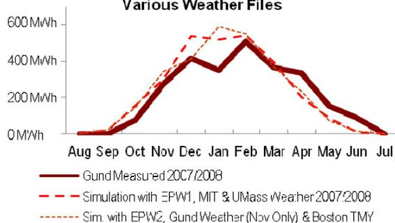
**Figure 5: Heating Load Comparing Weather Files**
