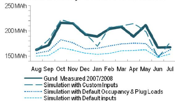
**Figure 6: Electricity - Measured vs. Simulations**
