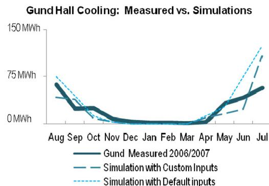
Figure 8: Cooling – Measured vs. Simulation
