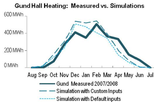
Figure 7: Heating – Measured vs. Simulations
