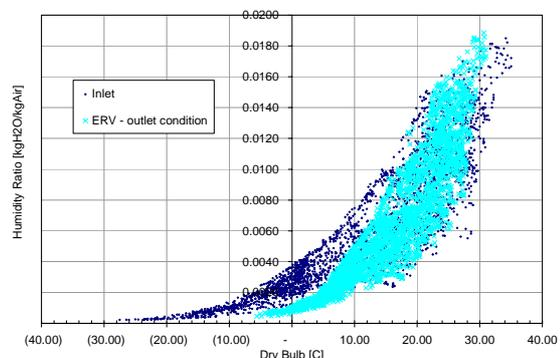
Figure 3: Inlet/Outlet Air Conditions (ERV pre-treatment)
