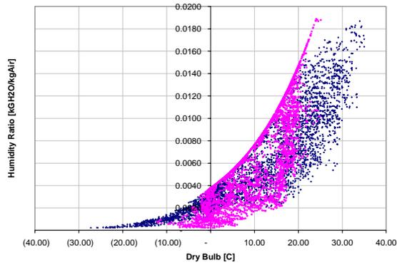
Figure 4: Inlet/Outlet Air Conditions (Earth Duct pre-treatment)
