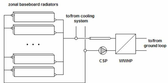
*Figure 1: Meeting Wing Heat Pump / Radiator Subsystem Schematic*
