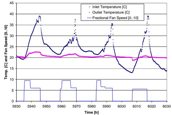
Figure 5: Measured Earth Duct Inlet and Outlet Conditions
