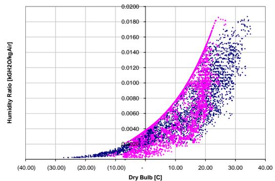
*Figure 7: Inlet/Outlet Air Conditions (Calibrated Earth Duct pre-treatment)*
