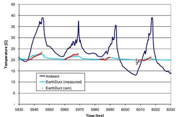
Figure 6: Measured and Simulated Earth Duct Outlet Temperatures
