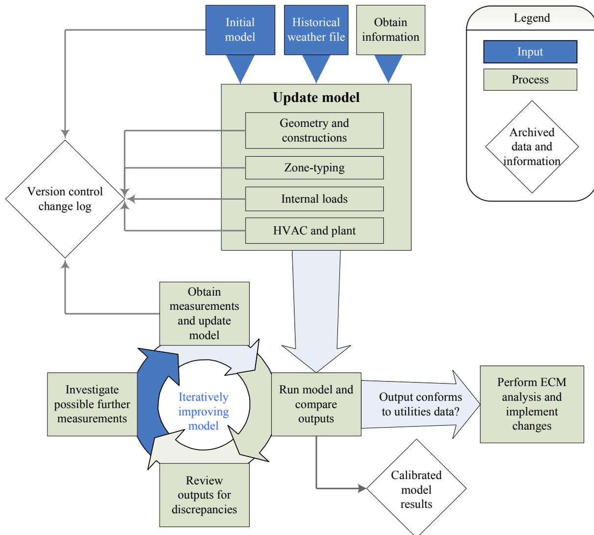
Figure 1 Calibration methodology
