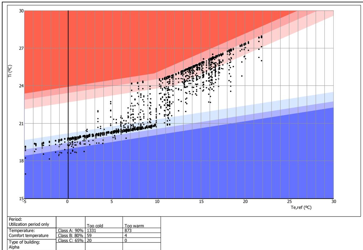
Figure 4: ATG-graph for the reference case (normal amount of fresh air, local cooling present)
