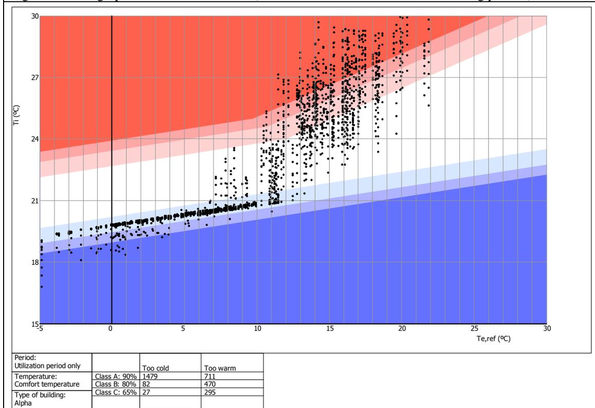
Figure 5: ATG-graph for the case with double ventilation rate
