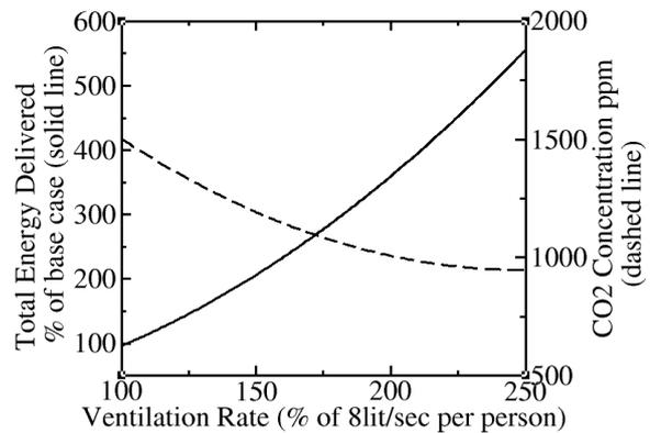
Figure 4 Energy use and CO2 concentration by ventilation rate
