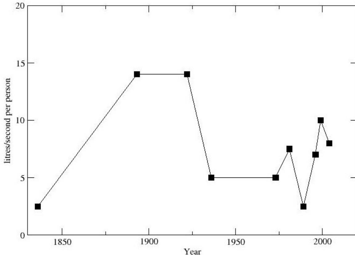
Figure 1 ASHRAE 62 (and equivalent) minimum fresh air requirements
