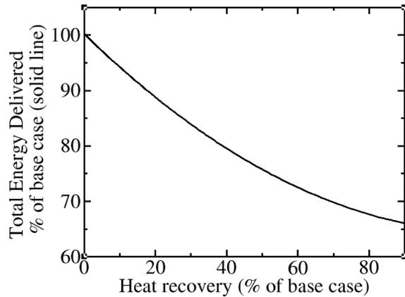
Figure 6 Energy use by heat recovery (same CO<sub>2</sub> concentration as base case)
