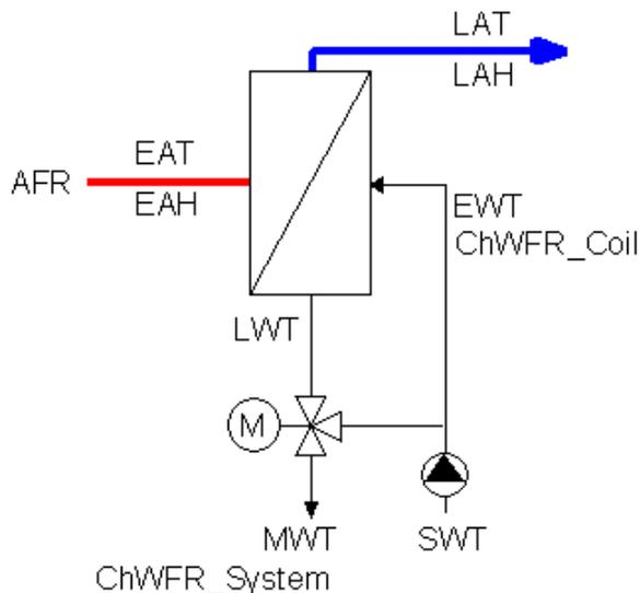
Figure 5 Coil with variable water flow rate
