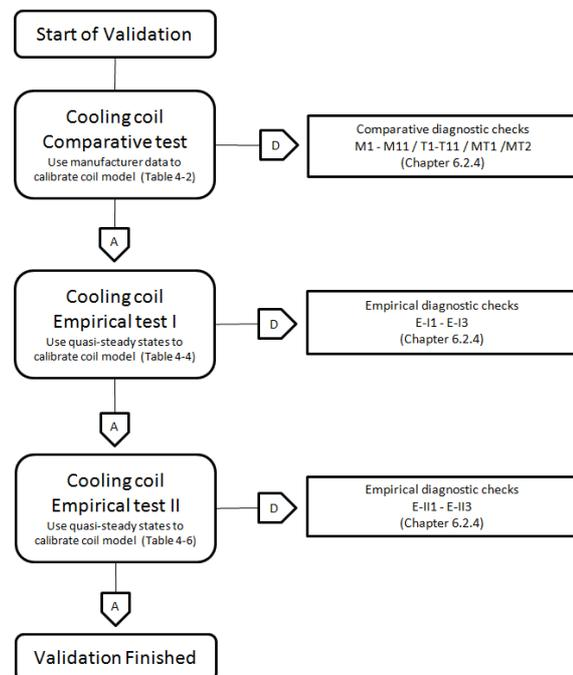
Figure 4 Cooling coil overall test logic
