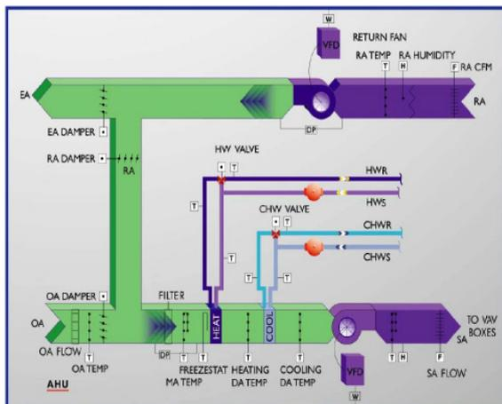
*Figure 1 Schematic plot of AHU system with measuring points*
