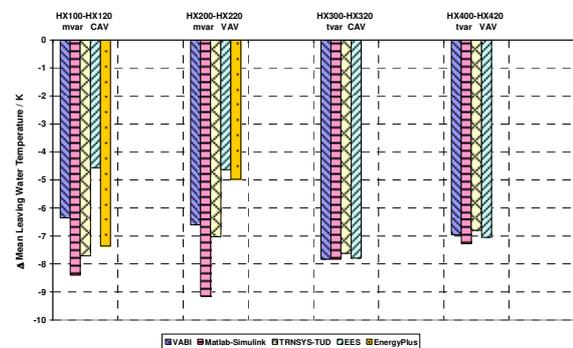
Figure 11 Sensitivity of mean leaving water temperature against leaving air temperature set point
