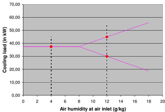
Figure 8 Cooling power (sensible and latent = total) for 2 points (1 in dry regime and 1 point in wet regime)
