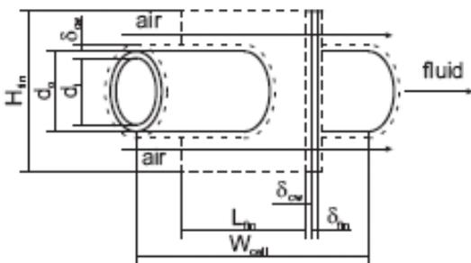
Figure 9 Sketch of a modelled cell as a part of a finned coil
