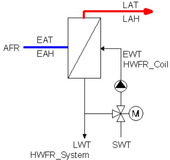
Figure 6 Coil with constant water flow rate
