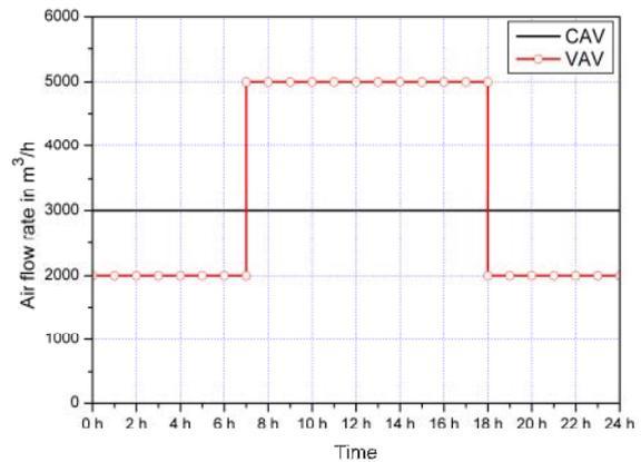
Figure 7 Air flow rate daily profile for cooling coil comparative testing
